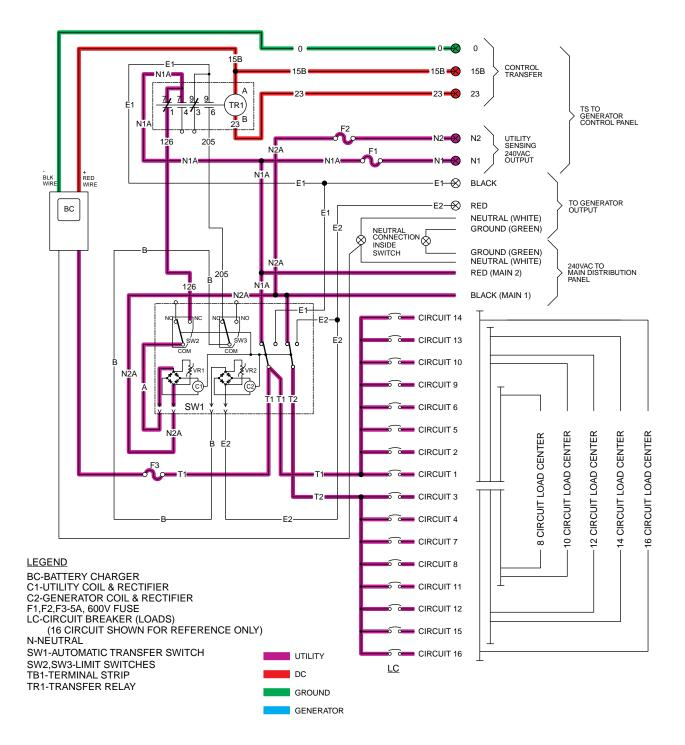
Figure 10. Transfer Switch in UTILITY.
